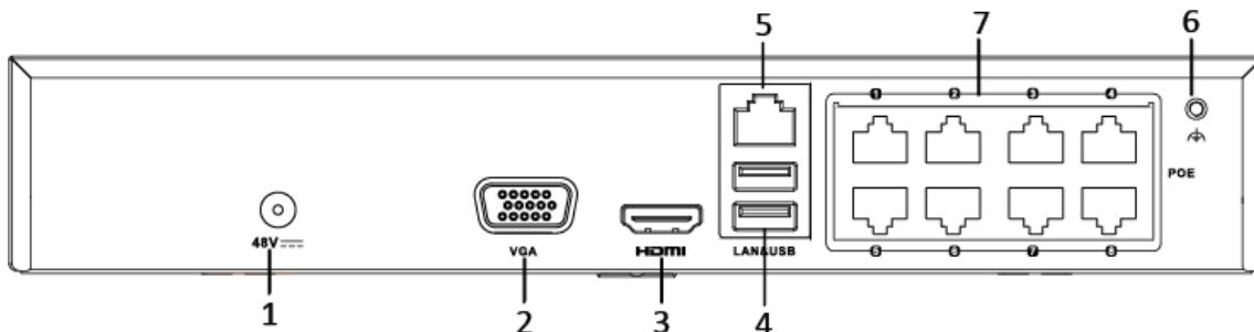
\*: The rear panel of NVR-104MH-D/4P provides 4 PoE interfaces.
